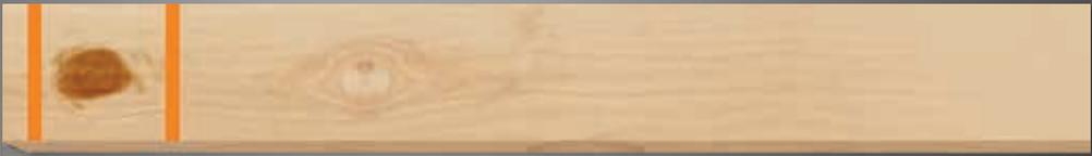
**\*Note: Crayon marks must be drawn a minimum of 36mm (1.41 inches) apart or MORE for defect marking.**
