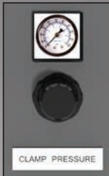
Adjusts the pressure of the horizontal and vertical clamps.
