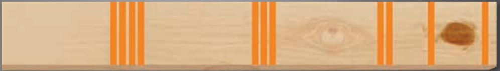
**\*Note: Draw two lines to tell your TigerSaw to move to Grade Marking List 1, three for Grade Marking List 2, and four for Grade Marking List 3.**
