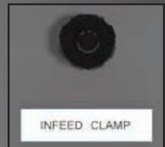
Adjusts the speed of the infeed clamps.
