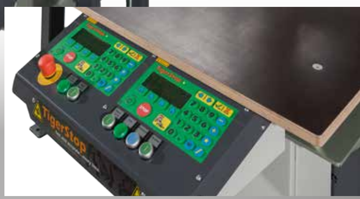
Automatic angle adjustment using TigerStop servo drive
