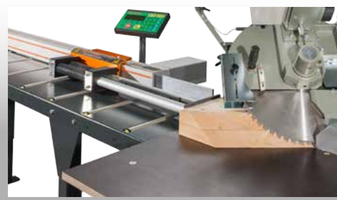
Automatic positioning with Tigerstop pusher system
