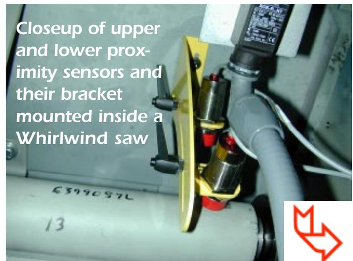
**Closeup of upper and lower proximity sensors and their bracket mounted inside a Whirlwind saw**
