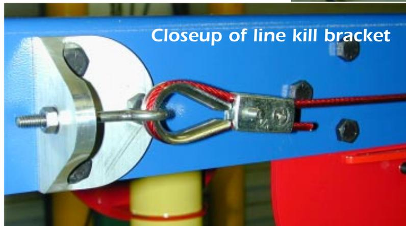
Mount the 1/4-20 eye bolt with cable thimble and cable clamp to the line kill bracket as shown in the picture to the left.
