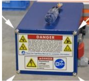
Fig. 5 - Using a 3/8" nut driver or socket to loosen and remove the 4 acorn nuts securing the motor box end cap.
