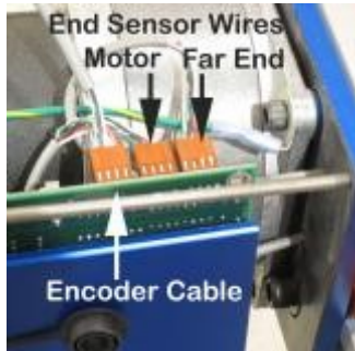
Fig. 7 - Disconnect the encoder cable and end sensor wires from the amplifier.
