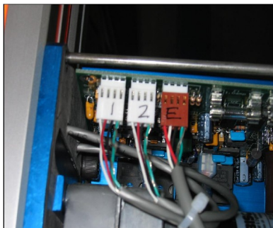
Fig. 13 - Connect the motor end sensor wire (the BOTTOM wire) to the contact marked Limit2.
