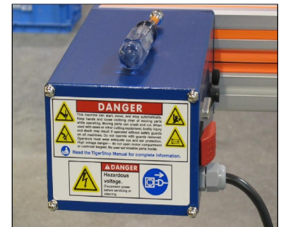
Fig. 15 - Fasten the motor box end cap over the stud bolts, thread the four acorn nuts on, and tighten them down.
