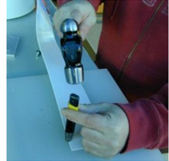
Fig. 17 — Punch the first hole.
