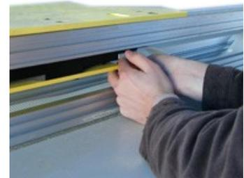
Fig. 21 — Clamp the end of the belt.
