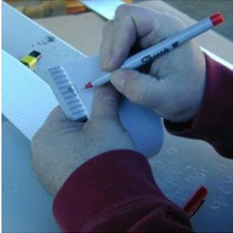
Fig. 15 — Mark first belt punch hole.
