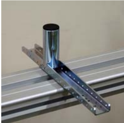
1. Place one plugged T-support on the saw stand.
