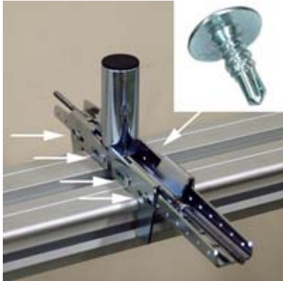
4. Place the T-support with the M-grips in position onto a work surface and drive 4 self-tap screws into the slotted holes of the M-Grips and into the round holes of the T-support on both sides. Tighten all 8 screws, then back them off half a turn. Return the assembly to the saw stand.
