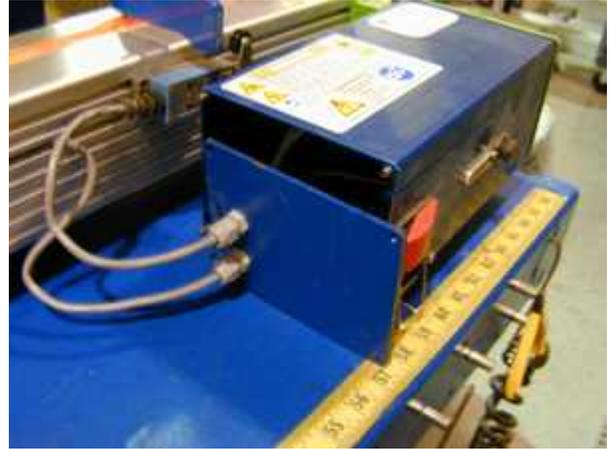
Pull the motor box end cap off the stud bolts. ▶
