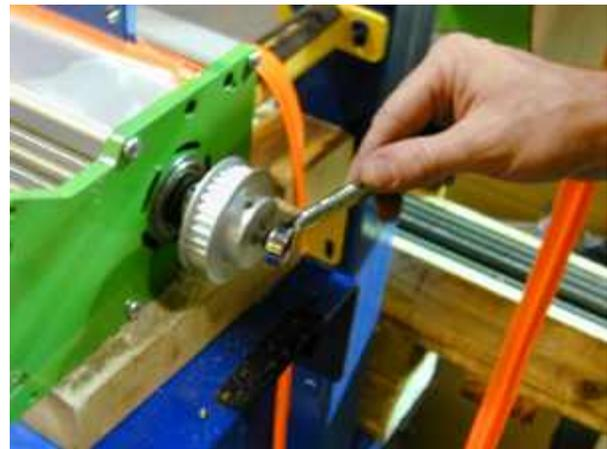
Reinstall the pulley, aligning the (2) set screws to the divots on the drive screw shaft, and tighten down with a 1/8" hex wrench. Screw the bolt into the end of the drive screw and fully tighten it with a 7/16" nut driver. ►
