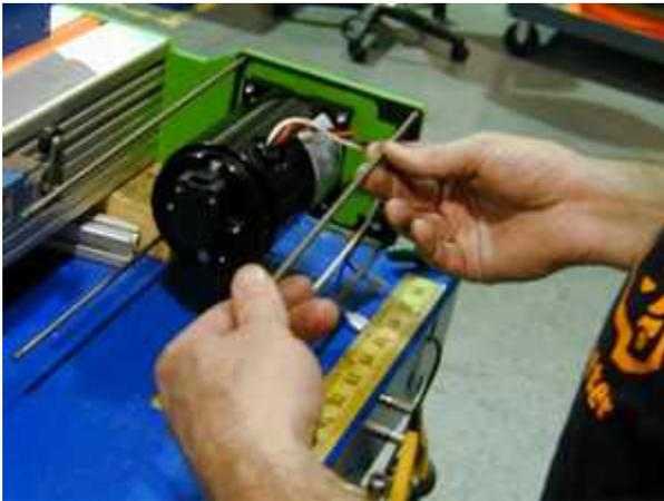
Screw the stud bolts into the motor end plate. ▶
