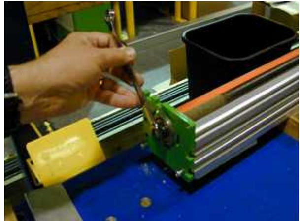
With a helper guiding the carriage at the motor end (**READ Caution below**), turn the drive screw anti-clockwise from the far end using a 7/16" wrench, so the carriage moves away from you until it is completely off the screw. ►
