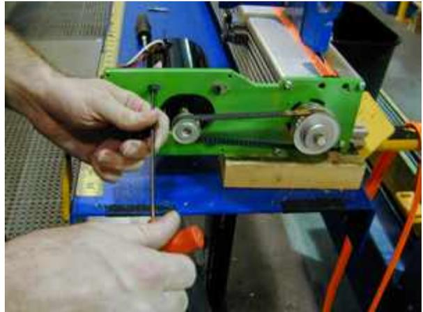
Using a 1/8" hex wrench, undo the (4) bolts securing the motor to the end plate. (On some models, use a 3/8" nut driver to remove these bolts.) ▶
