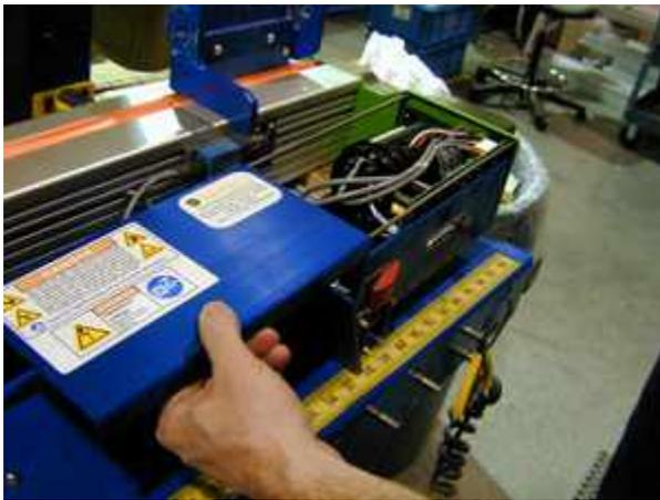
Slide the motor box cover off stud bolts. ▶
