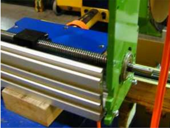
Reattach the motor end plate by means of the (2) lower screws, tightened partially, so the drive screw is supported. ▶
