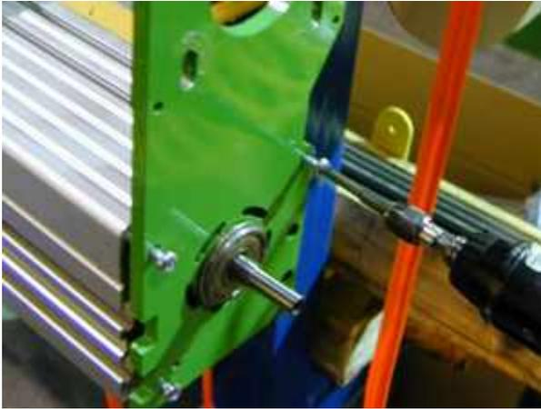
Insert the (2) top screws in the motor end plate, and partially tighten, using a T25 Torx driver. ►
