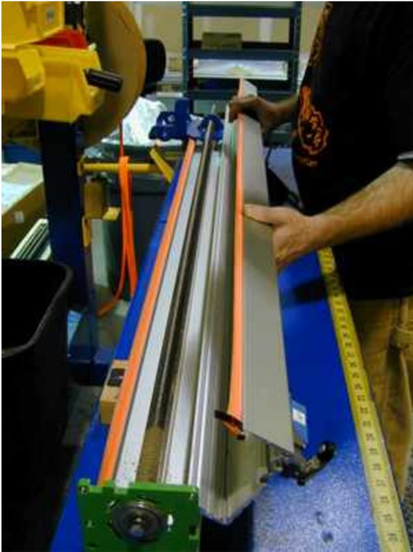
Firmly grasping the extrusion cover, pivot it towards you and carefully remove it. The drive screw is now totally accessible. ►
