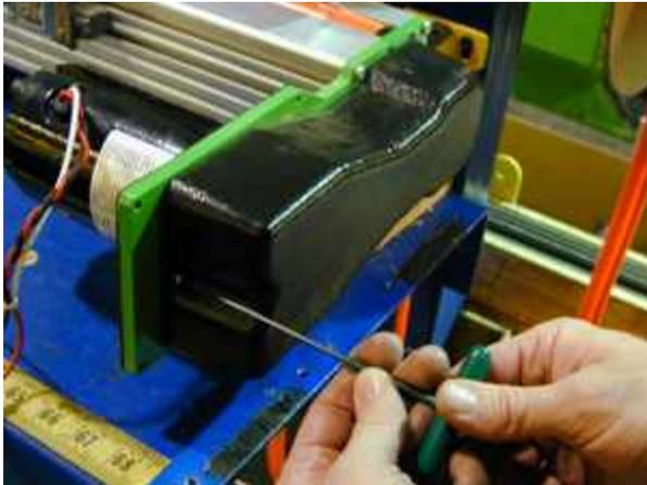
Using a 3/32" hex wrench, undo the (3) screws securing the drive belt cover, and remove it. ▶
