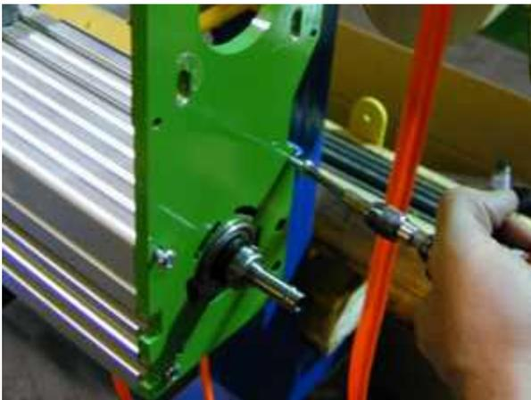
Finish tightening all (4) screws in the motor end plate, using a T25 Torx driver. Rotate TigerFence forward 90°. ►
