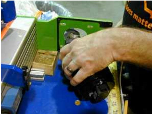
Remove the drive belt and motor. Clean out old silicone from the holes. ▶
