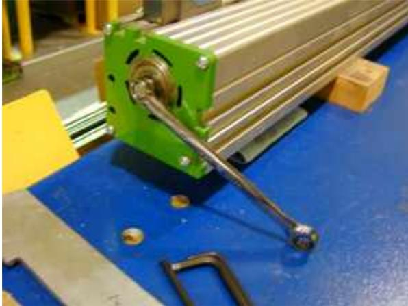
Use a 7/16" box wrench as a brake for the drive screw at the far end plate. ▶
