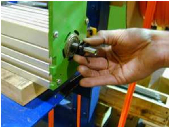
Remove the two washers from the drive screw. ▶
