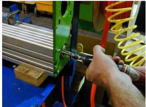
Using a T25 Torx driver, remove the (4) screws securing the motor end plate to the extrusion. ▶
