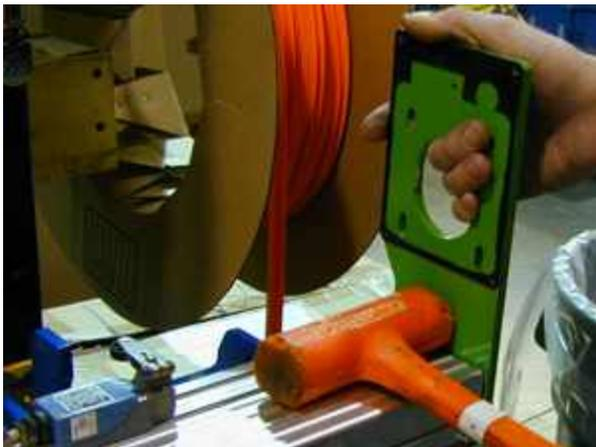
Using a dead blow mallet, tap the motor end plate loose from the extrusion and remove it. ▶
