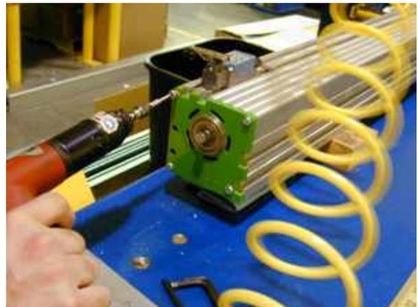
Using a T25 Torx driver, remove the top (2) screws securing the far end plate to the extrusion, and partially undo the bottom (2). ▶
