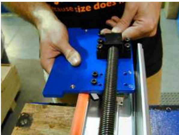
Thread the replacement carriage assembly back onto the drive screw. Turn the screw using a 7/16" wrench at the far end. ▶
