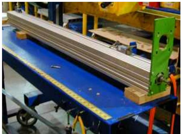
Carefully rotate TigerFence 90° so the motor end plate is standing straight up. ▶
