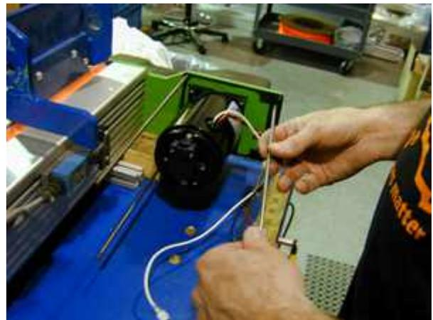
Remove the (4) stud bolts from the motor end plate. ▶
