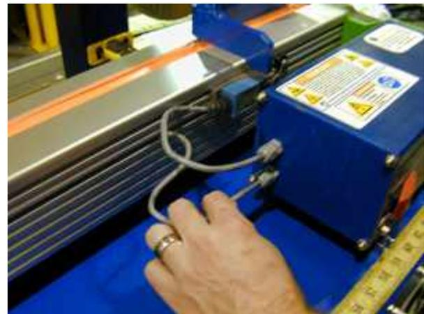
Carefully pull on the end sensor cables at the strain reliefs to make room to work, but do **not** pull them all the way out. ►
