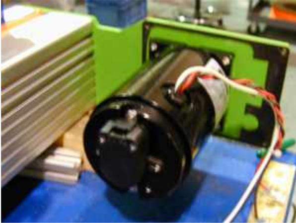
Mount the motor back onto the motor end plate using the (4) bolts, but do not tighten yet. Put the drive belt back on the (2) pulleys. ▶
