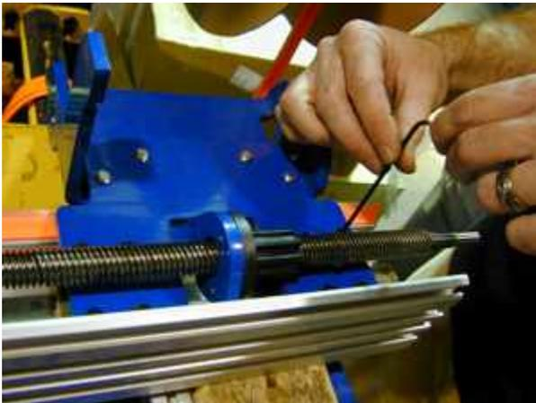
Using a 3mm hex wrench (or 8mm nut driver on existing hex head bolts), remove the (8) round head bolts securing the linear bearings. ►
