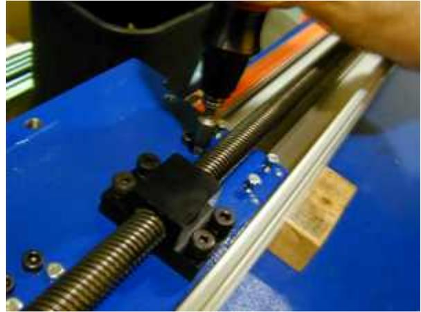
Using an 8mm nut driver, tighten the (8) bolts that secure the linear bearings. If you have a torque wrench, tighten them to 78 in-lbs. ▶
