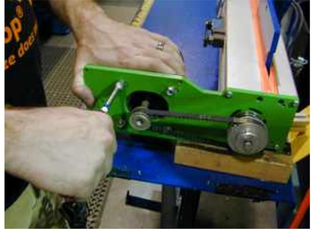
Pulling the motor away from the drive screw to add tension to the belt, fully tighten all (4) bolts securing the motor, using a 3/8" nut driver. ▶
