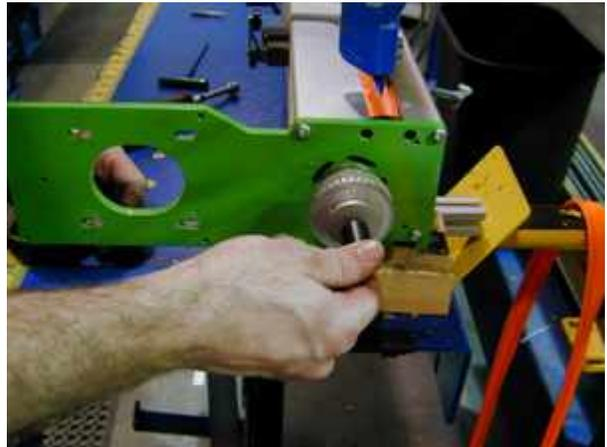
Using a 7/16" nut driver, remove the bolt from the end of the drive screw. ▶
