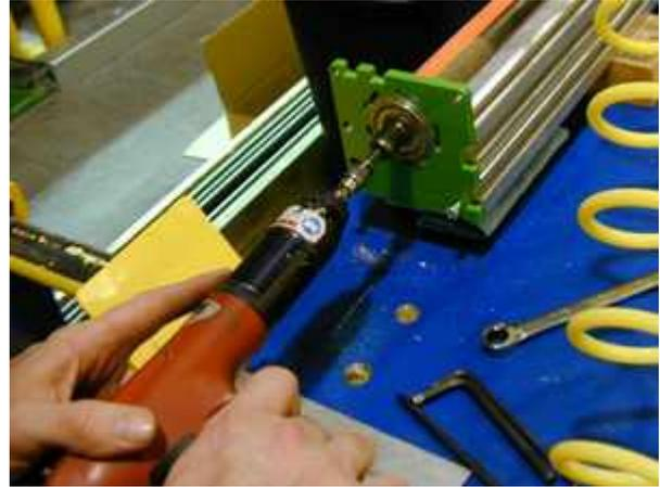
Using a power tool and a 7/16" nut driver, turn the screw from the far end till the carriage moves to about 1/2" from the far end plate. ▶
