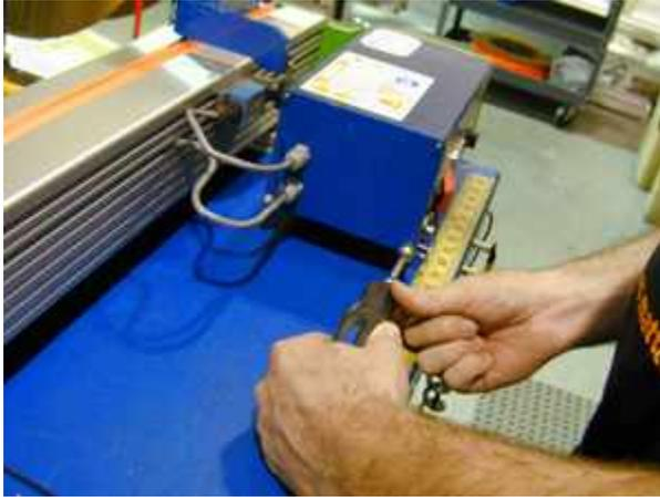
Using a 3/8" nut driver, remove the (4) acorn nuts from the motor box end cap. ▶
