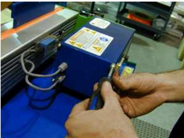
Press the motor box end cap onto the stud bolts, add the acorn nuts, and fully tighten them down, using a 3/8" nut driver. ▶
