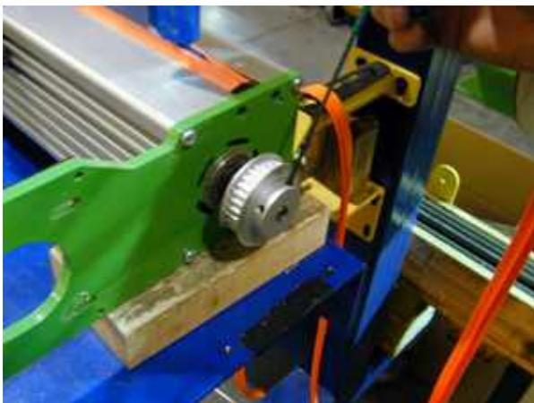
Using a 1/8" hex wrench, loosen (2) set screws securing the pulley to the drive screw, and remove the pulley. ▶
