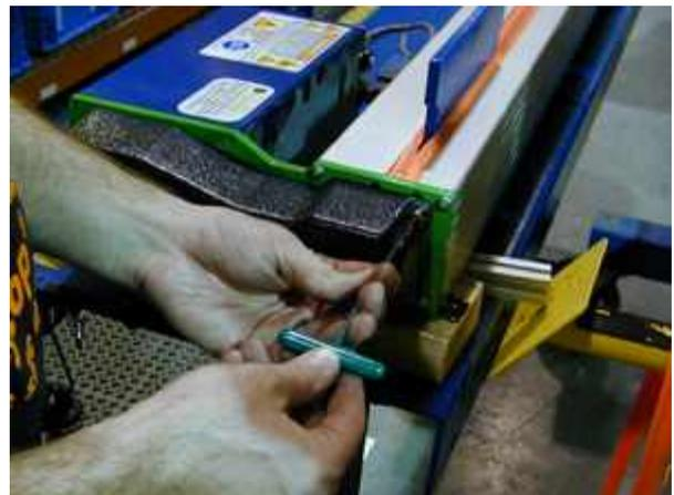
Re-install the drive belt cover and fully tighten the (3) screws securing it to the motor end plate, using a 3/32" hex wrench. ▶
