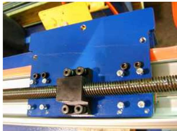
Line up the (8) holes in the carriage assembly with those in the linear bearings.
