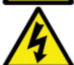
Do not open motor compartment or controller keypad. DC voltage with potentially **FATAL** amperage! Disconnect power before servicing.
